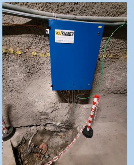
BHS-1 borehole with sensor lines and the green outflow pipe (top), IBC tank with bottom outflow pipe, gas extraction device
